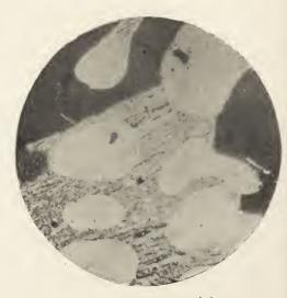
Fig. 26. Basic Pig Iron, containing 2.9 per cent. P. Structure developed by "heat tinting"—the dark flat areas are cementite.
